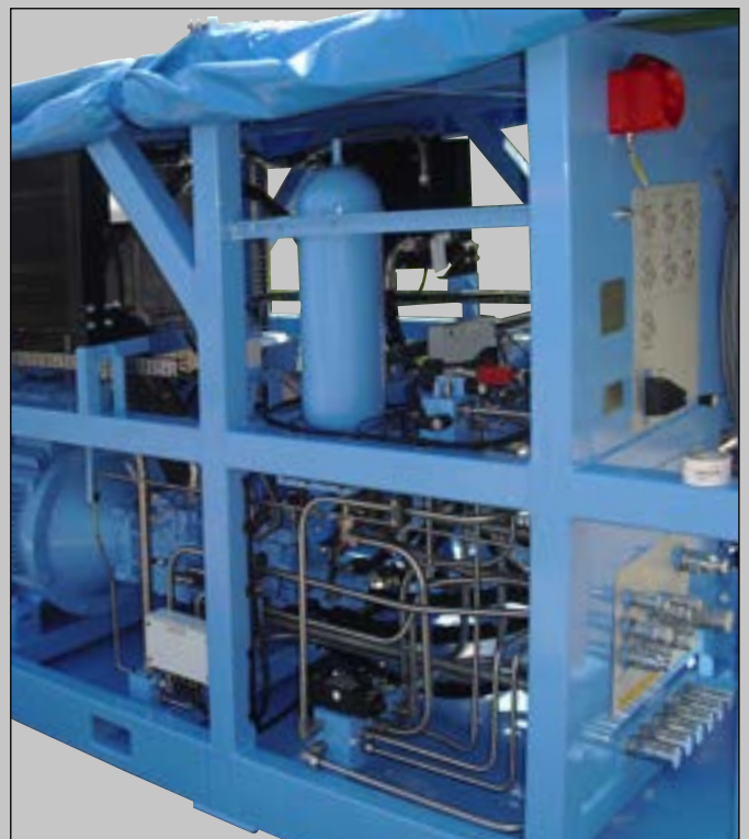
Marine, zone rated power unit suitable for containerisation
